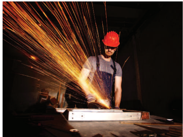
A stream of sparks from disc cutting
